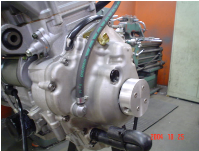
Our MCX turbo oil return pump is used on the Nytro FX. The photo shows the pump installed on the RS engine.
