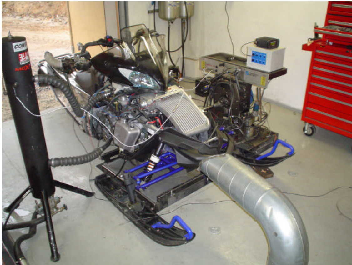
Yamaha Apex rear mount turbo during dynotest in our SF 901 dyno. Note the external cooling tower. The engine water temperature is stable even if you run the engine at full power for several minutes.
