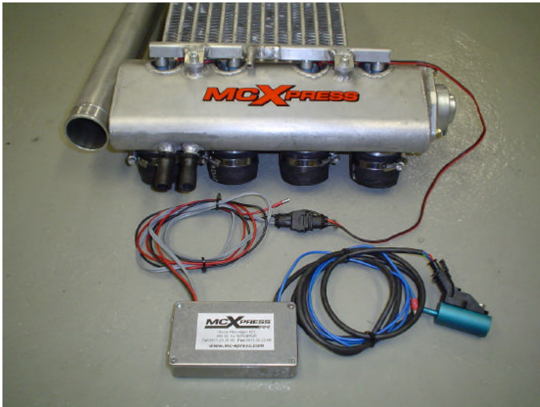
MCX EFI-box with Map-sensor and Apex intercooler / plenum
